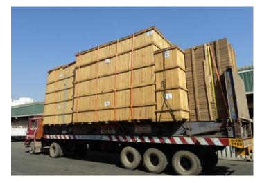
Trailer systems are intensively used in conjunction with other machinery for lifting and transporting heavy goods. They are generally integrated with large trucks to move cargo efficiently and quickly.
